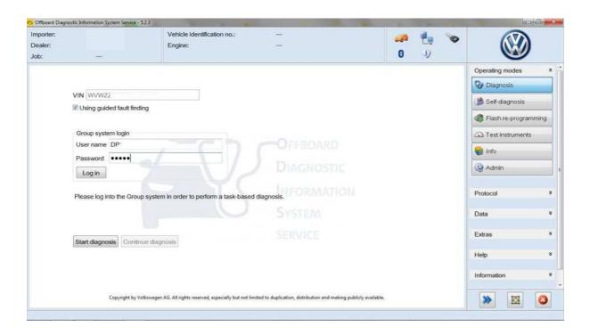
After this log in, necessary SFD activation tokens for work on the control units are generated automatically in the background.
