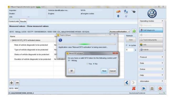
The activation request structure generated by the control unit is required so that the SFD back end can generate an activation token. You can now either copy the structure to the clipboard or save it in a file:
